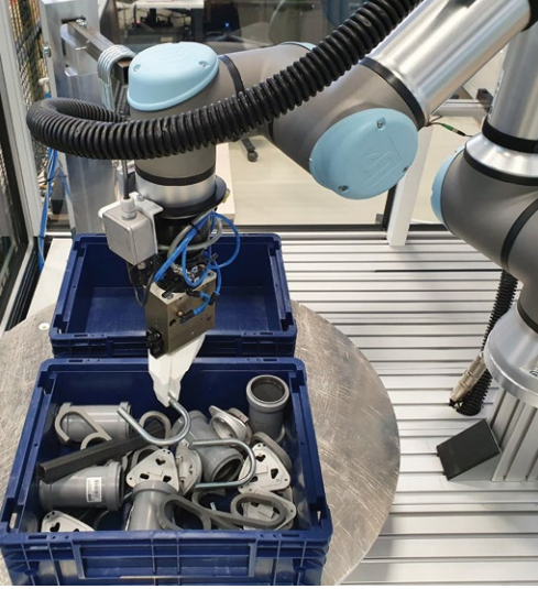
Picking different workpieces out of a mixed bin (left).
