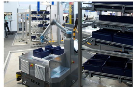
Replenishing small load carriers in the production warehouse with a mobile manipulator.
